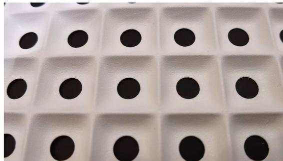
吸塑样品对应LED pitch~10mm.
